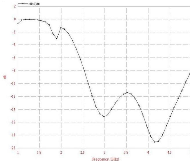
Fig.3. Return loss v/s frequency graph.
