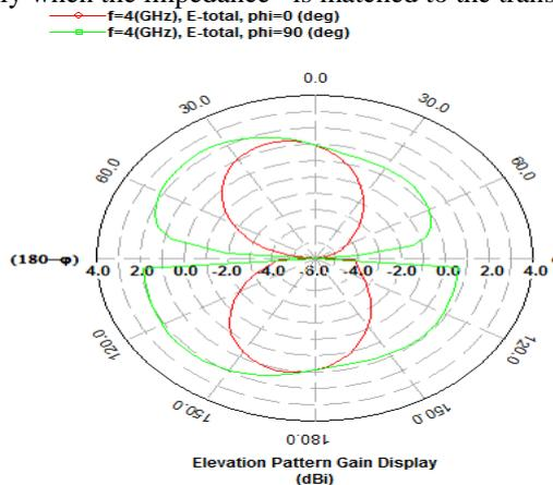
Fig.6. 2D pattern of proposed antenna
