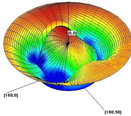
Fig.4. 3D Radiation pattern of proposed antenna..
