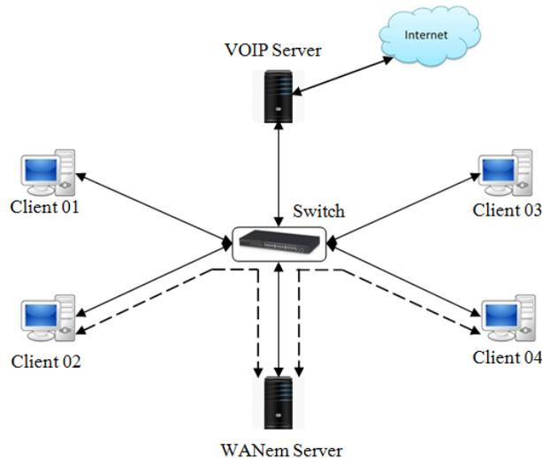
Figure 02: Network setup to get degraded signal
