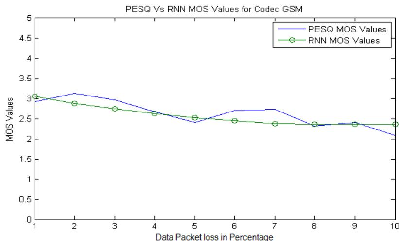
Figure 05: PESQ Vs RNN MOS using codec GSM
