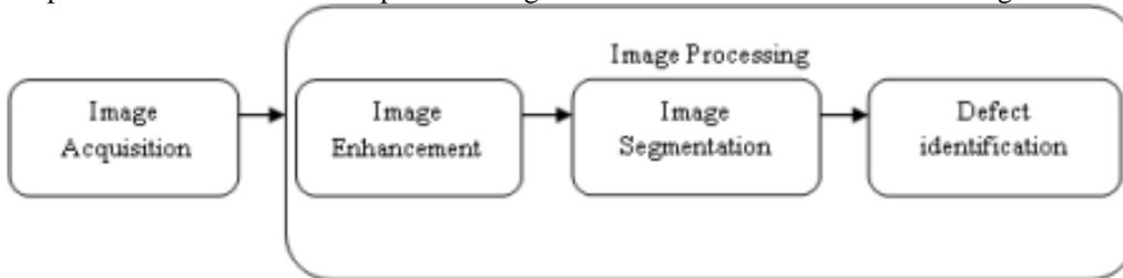
Fig 1 Methodology of Defect Detection
