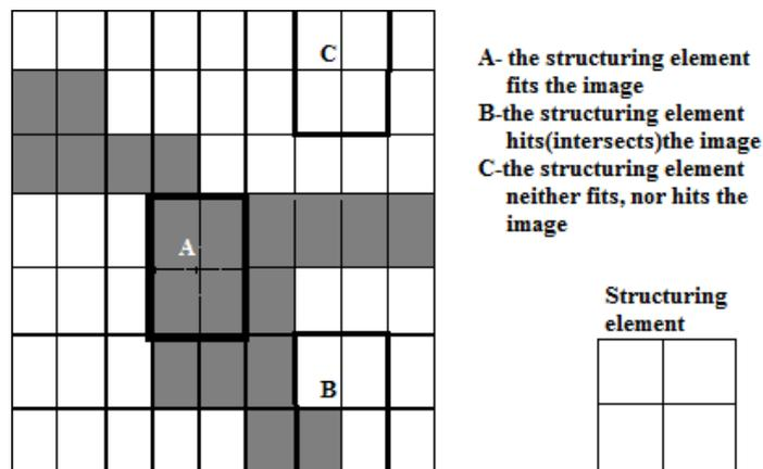
Fig.2 Probing of an image with a structuring element
