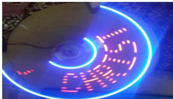
Fig. 7: Persistence of Vision at 600 RPM
