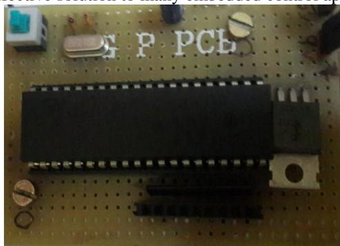
Fig. 1: AT89S53 micro-controller mounted on a PCB
