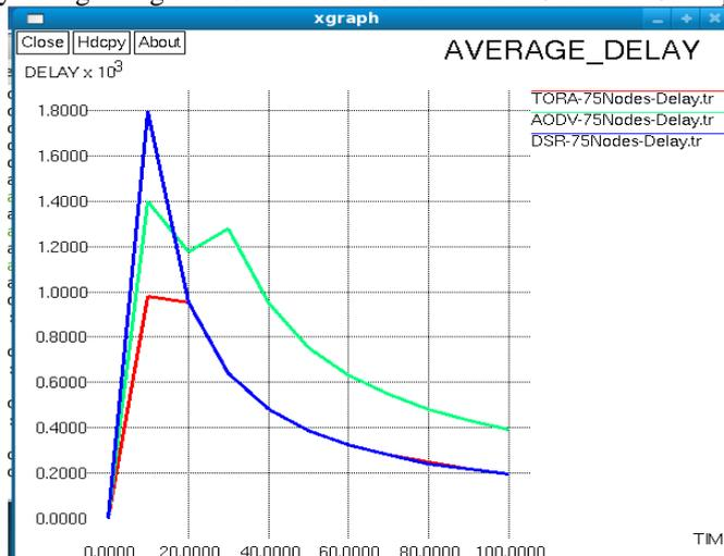
Figure: Average Delay Comparison of DSR, AODV and TORA for Network Size 75-Nodes
