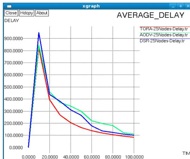
Figure: Average Delay Comparison of DSR, AODV and TORA for Network Size 25-Nodes
