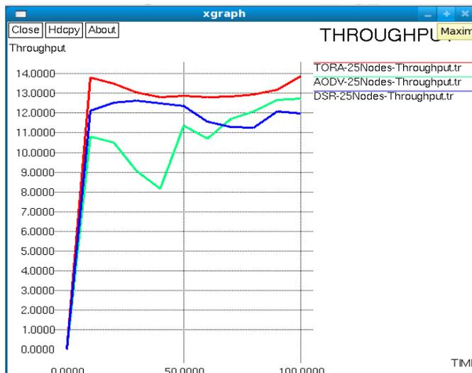
Figure: Throughput Comparison of DSR, AODV and TORA for Network Size 25-Nodes
