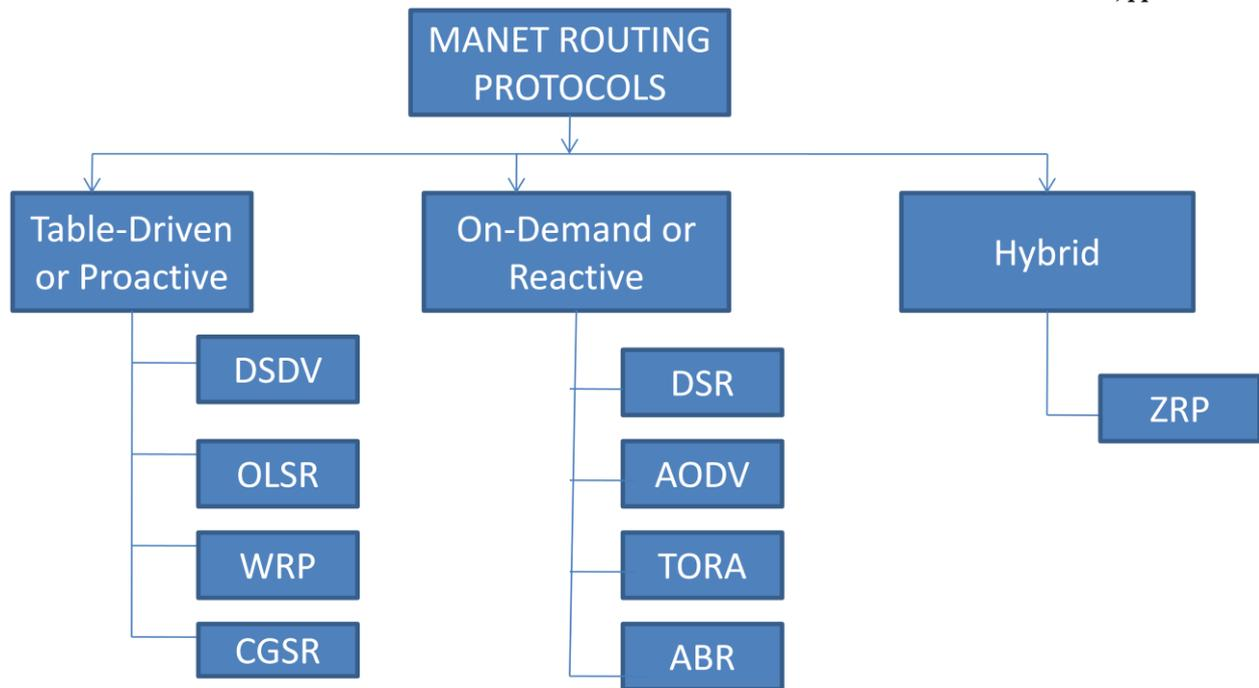
Figure: classification of MANET routing protocols.
