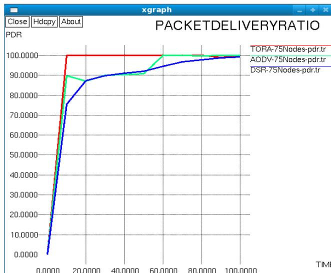
Figure: PDR Comparison of DSR,AODV and TORA for Network Size 75-Nodes
