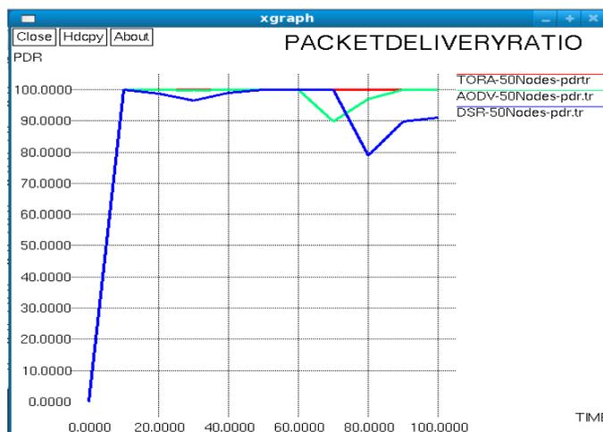
Figure: PDR Comparison of DSR, AODV and TORA for Network Size 50-Node
