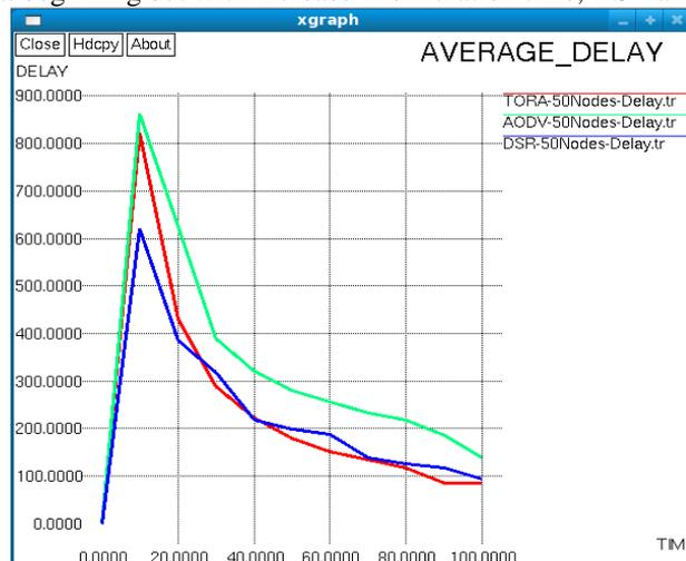
Figure: Average Delay Comparison of DSR, AODV and TORA for Network Size 50-Nodes
