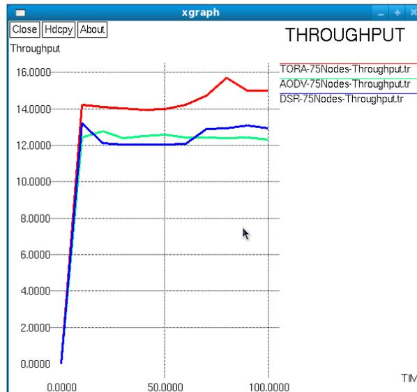
Figure: Throughput Comparison of DSR, AODV and TORA for Network Size 75-Nodes
