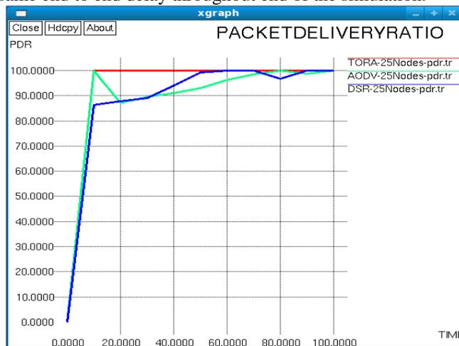
Figure: PDR Comparison of DSR, AODV and TORA for Network Size 25-Nodes
