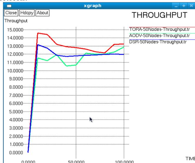
Figure: Throughput Comparison of DSR, AODV and TORA for Network Size 50-Nodes
