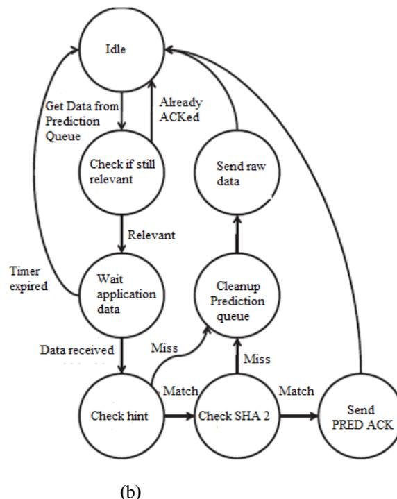
Figure 2. Sender algorithms. (a) Filling the prediction queue ,(b) Processing the prediction queue
