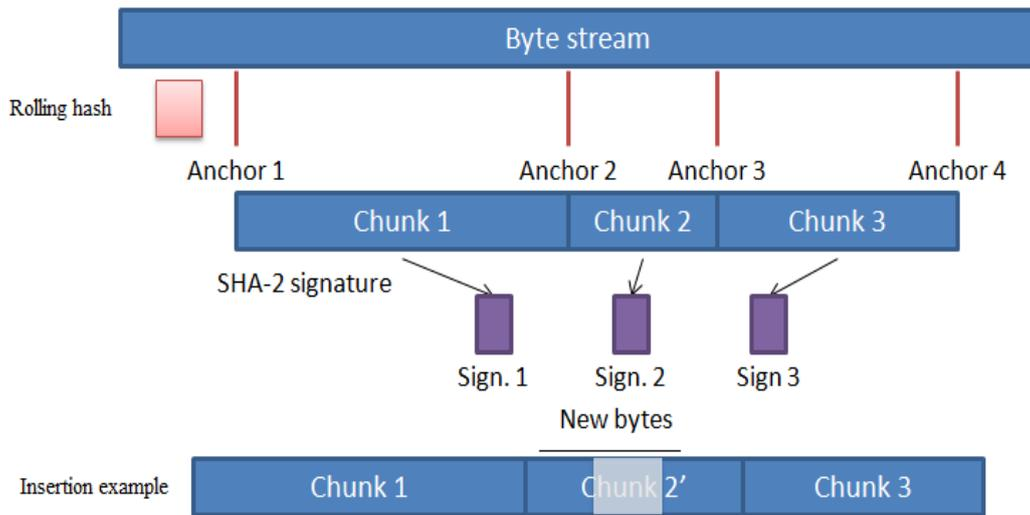
Figure 3. Server parses the outgoing stream to content-based chunks and signs with SHA-2.
