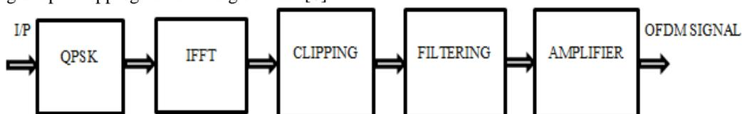
Fig.2. OFDM signal transmission block diagram
