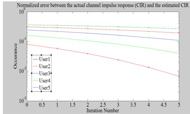
Fig 3. normalized error between actual CIR and estimated CIR
