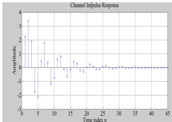
Fig 1.Channel impulse response
