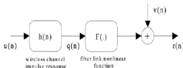
Fig-Fiber-wireless uplink modeled as a wiener system.
