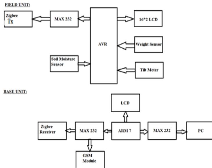
Fig. 3 Block Diagram of System
