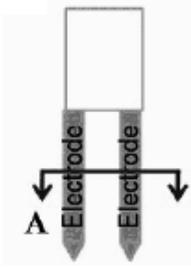
Fig.1 Soil Moisture Sensor
