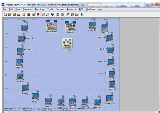
Fig: 1 Scenario with 20 WMN nodes with AODV protocol Implemented
