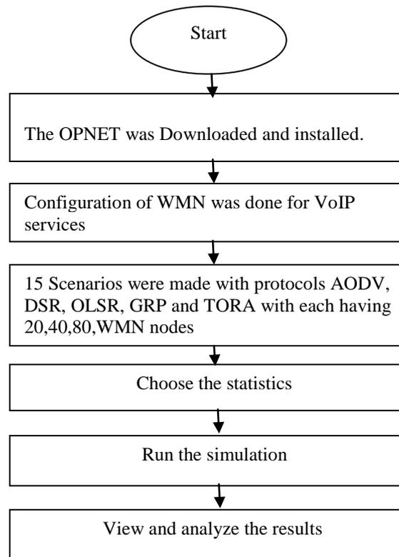
Fig:2 Flow Chart for simulation
