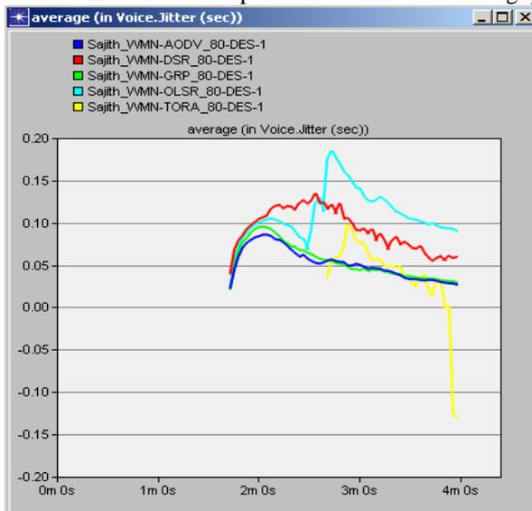
Fig:11 Showing Jitter value for 80 nodes
