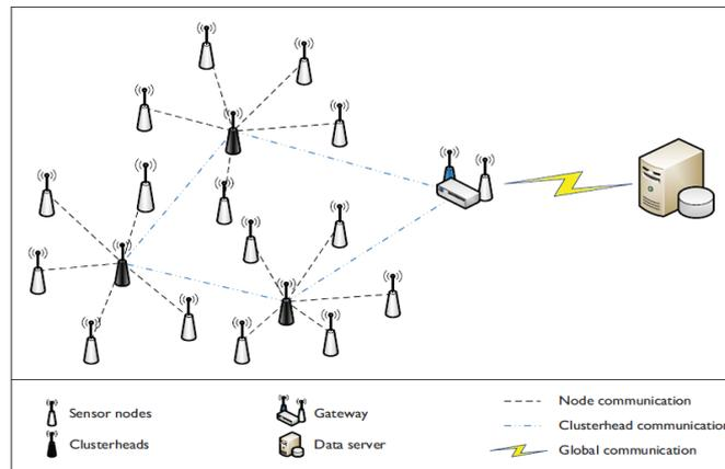
Fig. 1. Typical network architecture of environmental monitoring applications under scope
