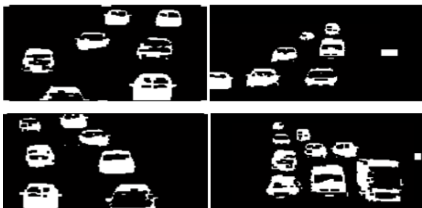
Fig.4 Moving vehicles detection using background subtraction method
