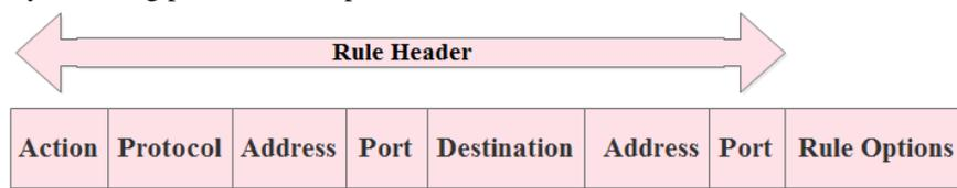
Fig. 6. Structure of a Snort rule.
