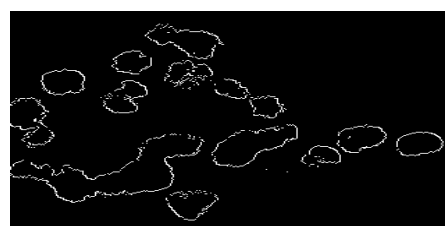
Fig.7. Trace of Gold nanoparticles 20nm for its shape measurement in TEM image
