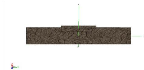
Fig.3 Parallel L-plate Feeding Differentially driven patch antenna in POSTFEKO
