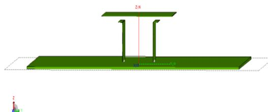
Fig.2 Parallel L-plate Feeding Differentially driven patch antenna in CADFEKO
