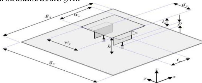
Fig.1 Geometry of Parallel L-Plate direct-feeding differentially driven patch antenna
