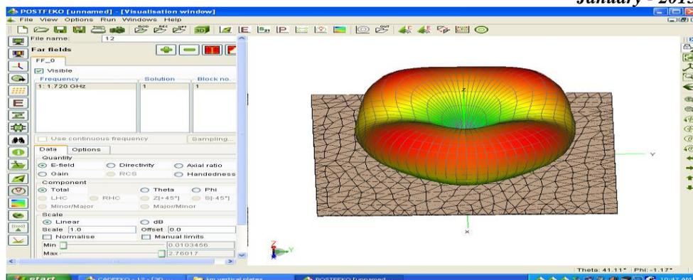
Fig.7 3-D view of radiation pattern
