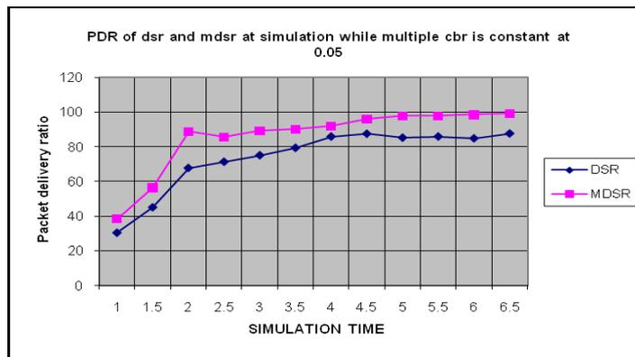
Figure 4: Packet delivery Ratio vs. Simulation Time
