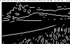
Fig. 10 Edge detection using Upper Constructor with laplacian operator
