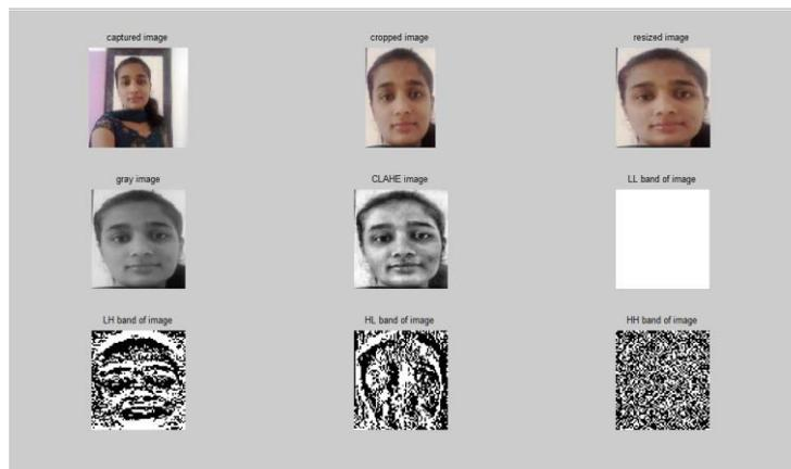
Fig 3.1. Simulation result of face detection, crop resize, CLAHE and DWT unit
