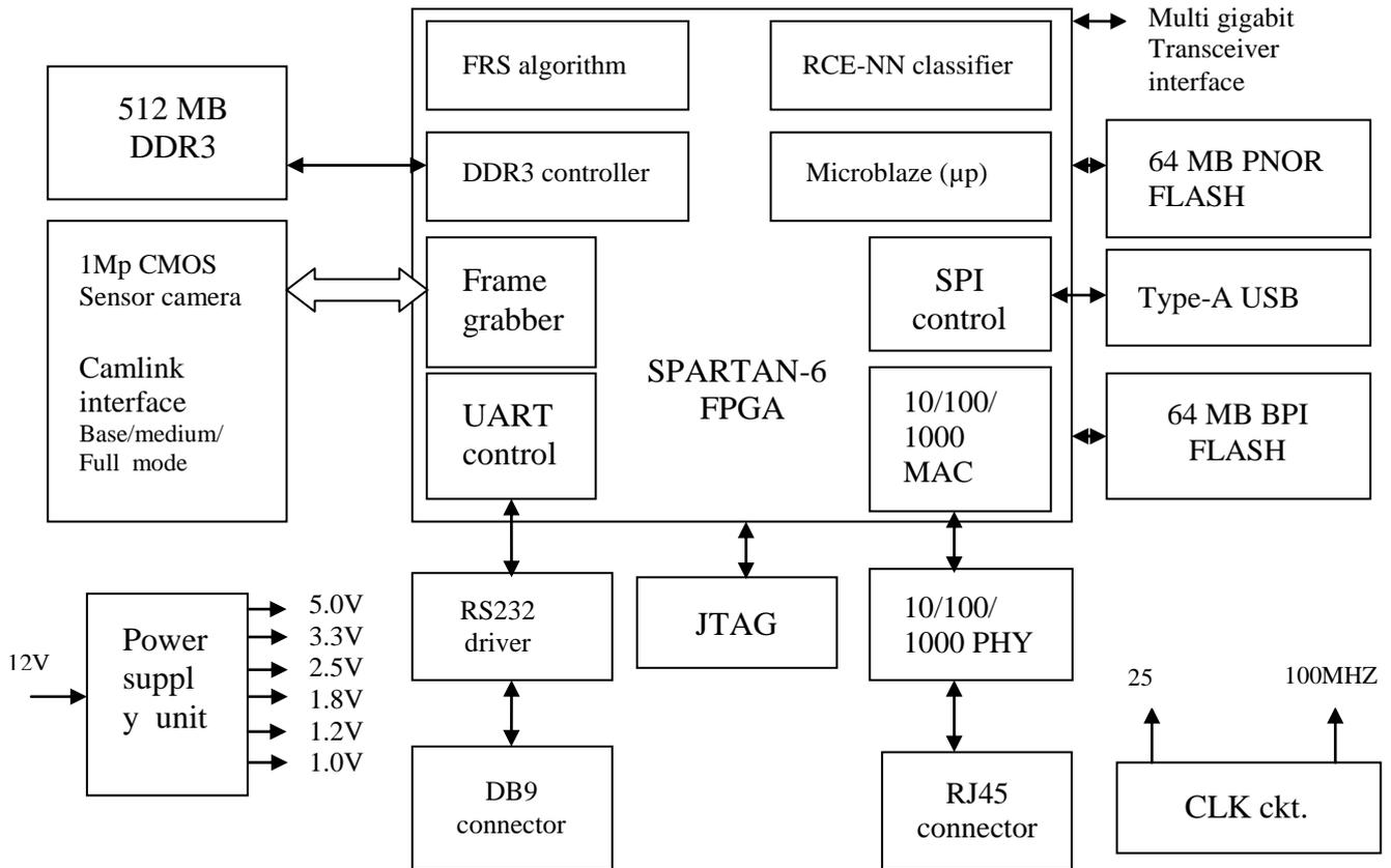
Fig 2.2. System hardware architecture block diagram
