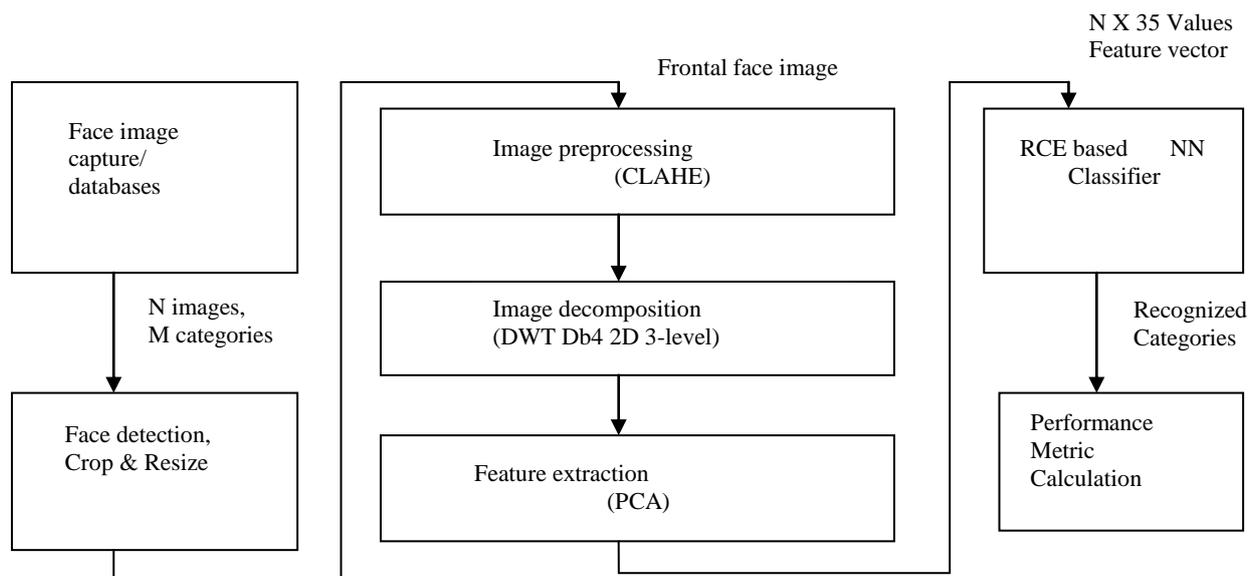
Fig 2.1. System overview block diagram
