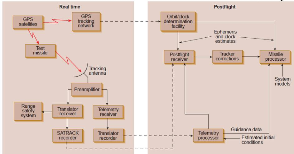
Fig. 1 Satrack configuration
