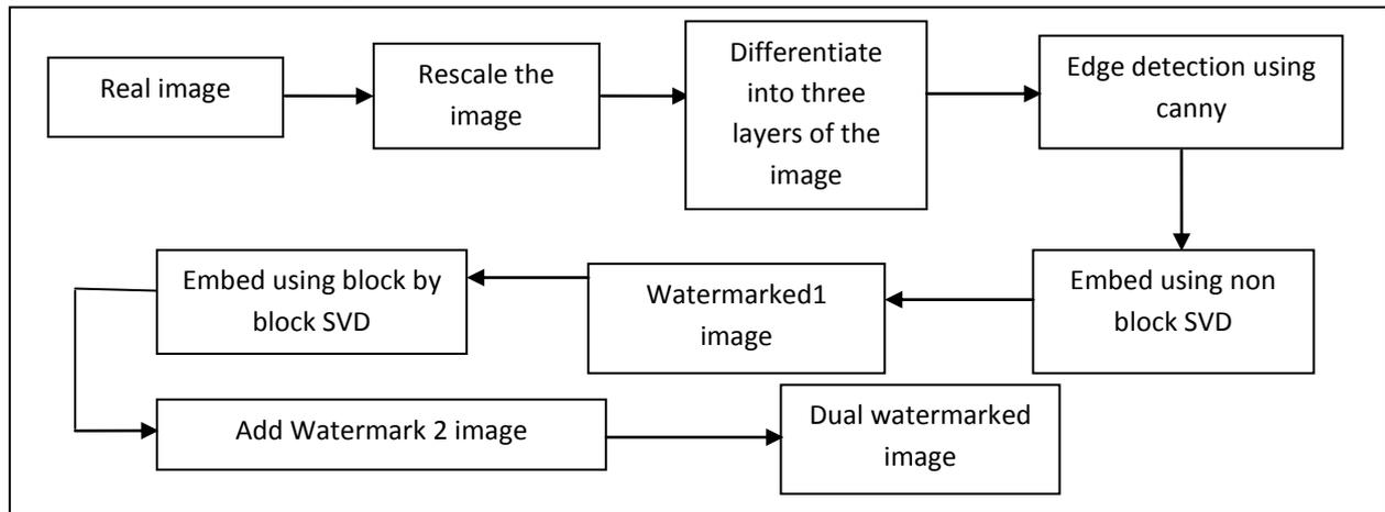
Fig 1. Block Diagram for Embedding Process
