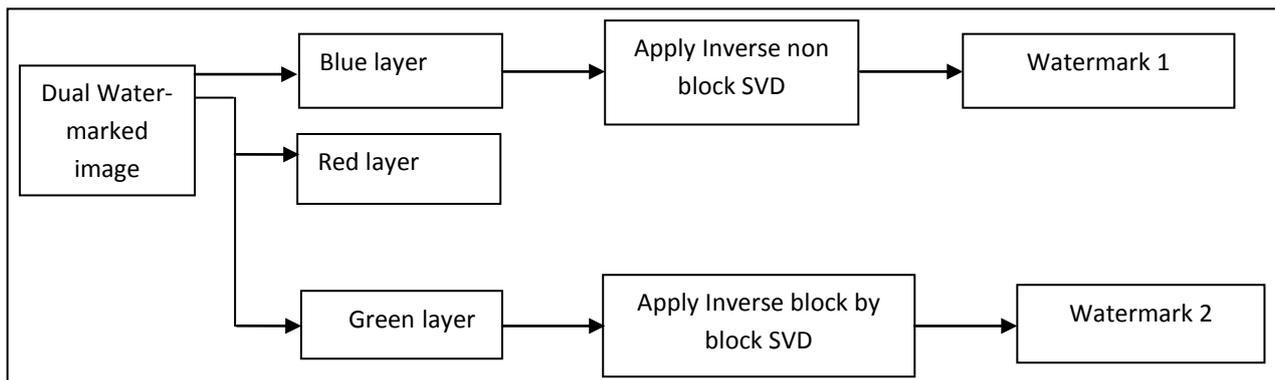
Fig 2. Block Diagram for the Extraction Process
