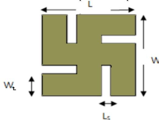
Fig.1.Swastik shape patch antenna [4]
