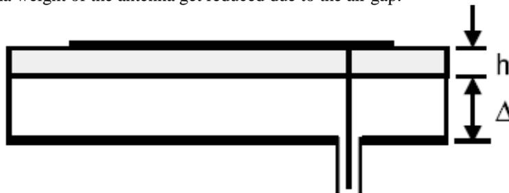
Fig.3. Suspended Antenna[6]
