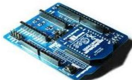
Fig: 3 Bluetooth mounted on wireless shield
