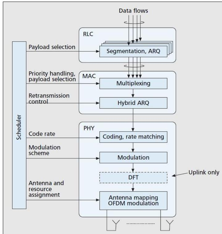
Fig. 4: LTE Protocol Structure (simplified) [6]
