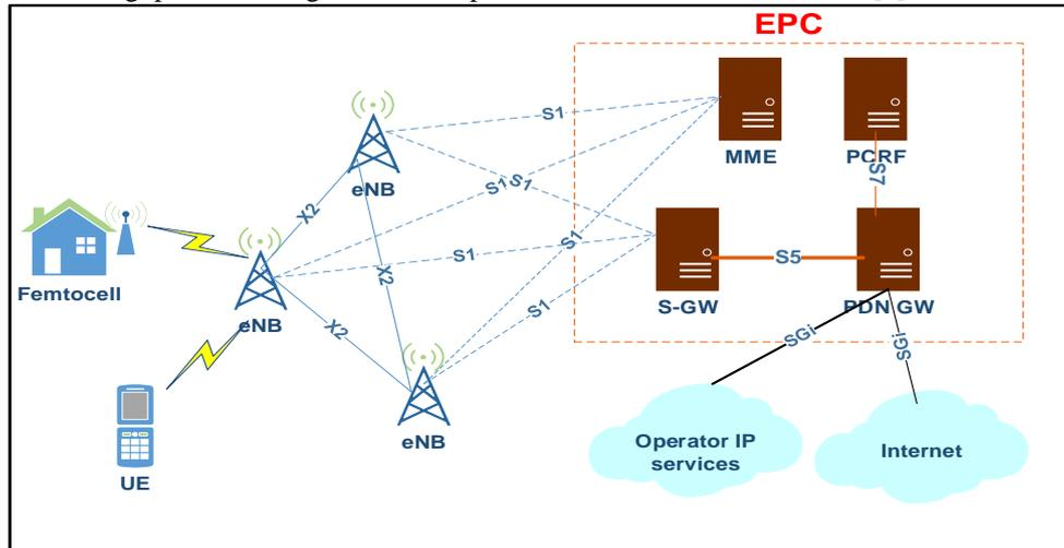
Fig. 5: LTE-Advanced Network Architecture.
