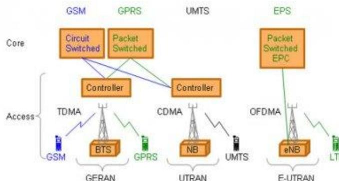
Fig. 3: Radio Access Network solution from GSM to LTE [4]
