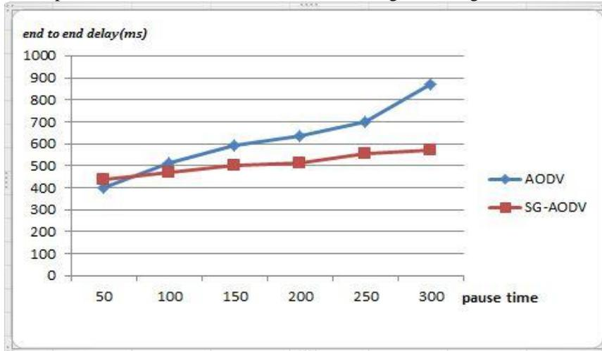
Fig. 6 End to End Delay of Protocols for 10 Nodes
