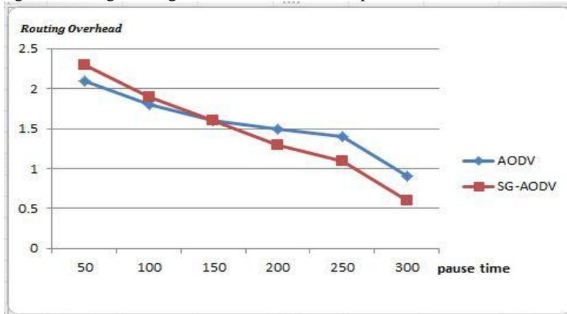
Fig. 10 Routing Overhead of Protocols for 10 nodes
