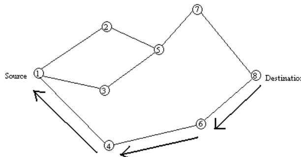
Fig. 3 Path Taken by Route Reply (RREP) Packet
