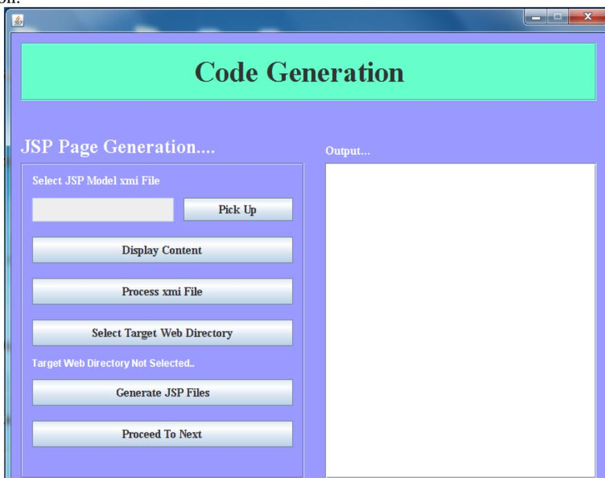
Fig. 4 JSP code generation form used to generate JSP pages where input is an XMI file
