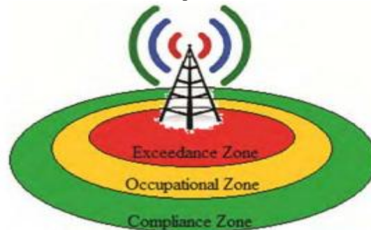
Fig.2: Marking of different zones around a base station antenna
