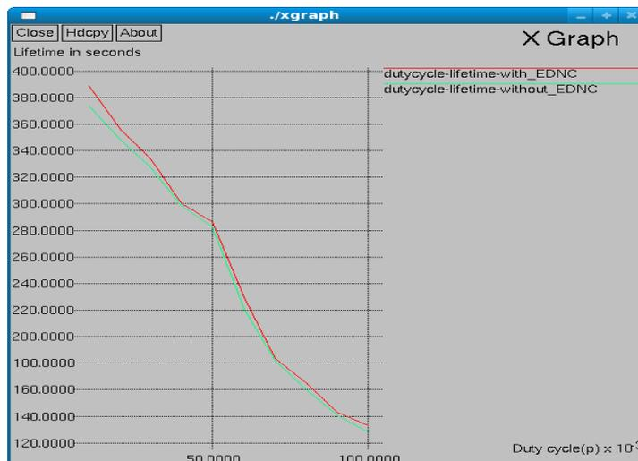
Figure. 2. Average network lifetime with duty cycle
