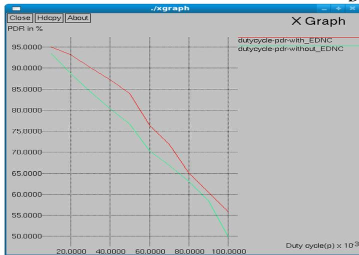
Figure. 3. Average packet delivery ratio with duty cycle
