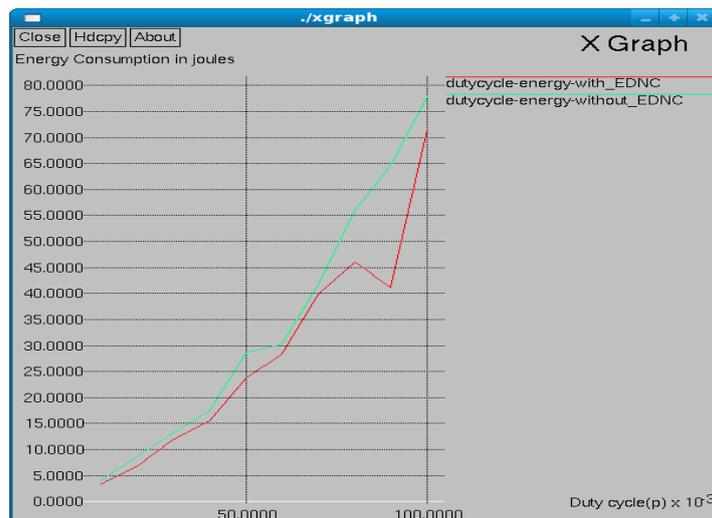
Figure. 1. Average energy consumption with duty cycle
