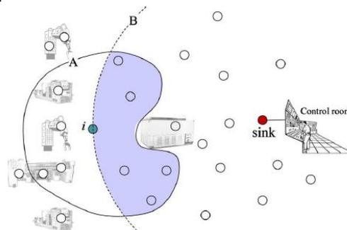
Neighboring nodes in Routing Table of node *i* in WISNs for manufacturing machines
