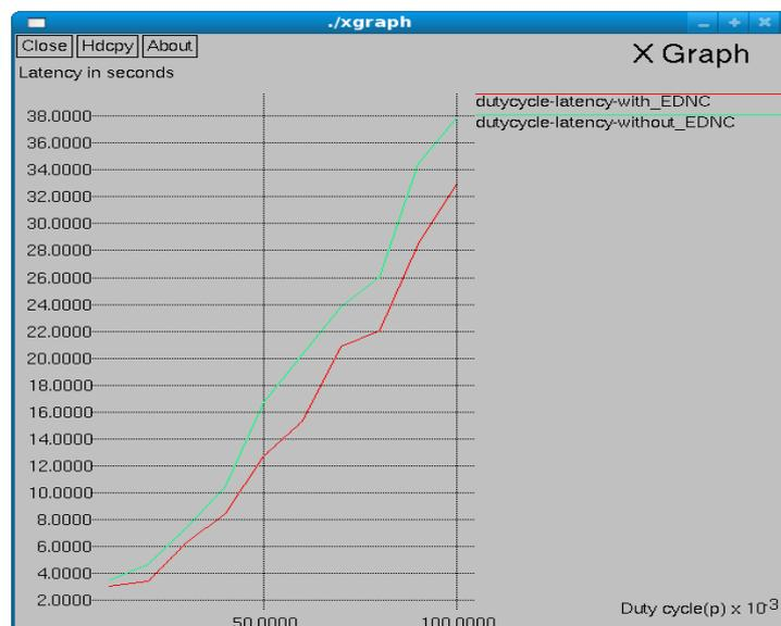
Figure. 4. Average latency with duty cycle
