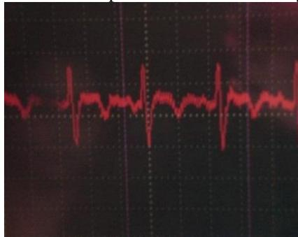
Figure 9. ECG signals achieved by the circuit as displayed on the digital oscilloscope
