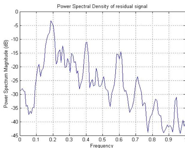
Fig 4(b):- Power spectral Density for residual noise signal (ANR ON)
