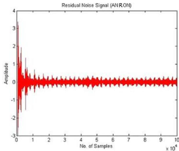
Fig 3:- The residual noise signal (ANR with secondary path modeling is ON)
