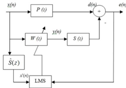
Fig 1:- FxLMS based ANR system.
