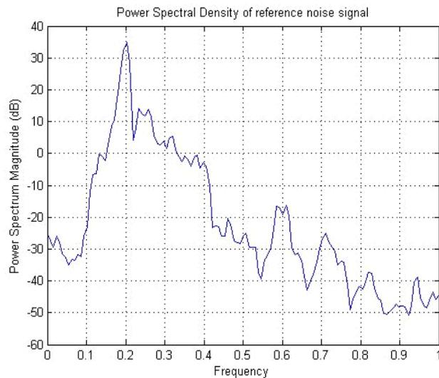
Fig 4(a):- Power spectral Density for reference noise signal of the ambulance siren noise (ANR OFF)
