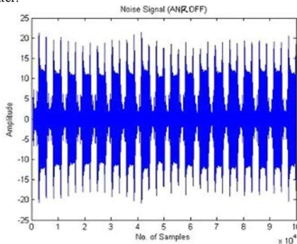
Fig 2:- The Ambulance Siren Signal taken as reference noise signal (ANR OFF)
