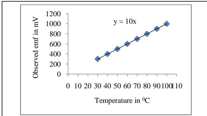
Figure.6 Graph of observed emf  $V_t$  (mV) against applied temperature  $t$  ( $^{\circ}\text{C}$ )
