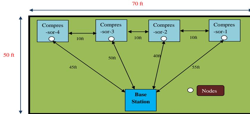
Figure 15 The Layout of the Refrigerator Section at Shivamruth Doodh Udadapak Sangh Maryadit.
