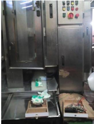
Figure 20 The Experimental Arrangement of the Wireless Sensor Network at Milk bag filling site.
