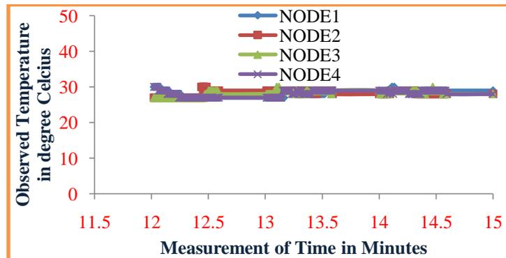
Figure 16 The Graph of Temperature values Measured at External Environment of Refrigerator Section against time in minutes
