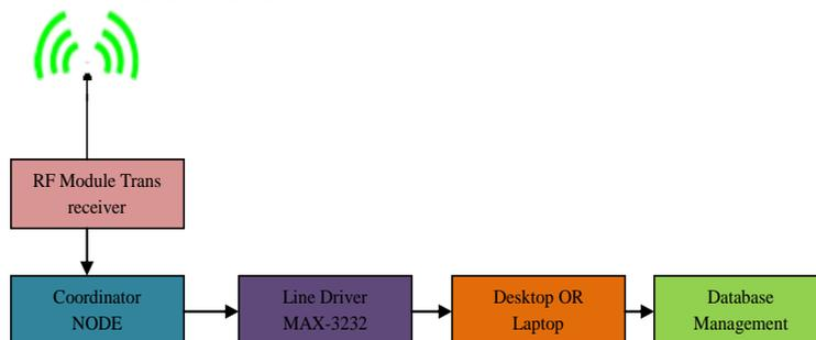
Figure.4 Block Diagram of Base Station with Coordinator
