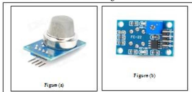
Figure 3 a) Front side of FC-22-I ammonia gas sensor module and b) the back side of FC-22-I sensor module
