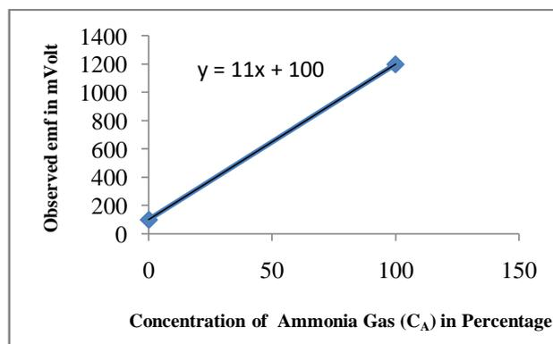
Figure. 7 Graph of observed emf  $V_A$  (mV) against Concentration of Ammonia Gas (%)
