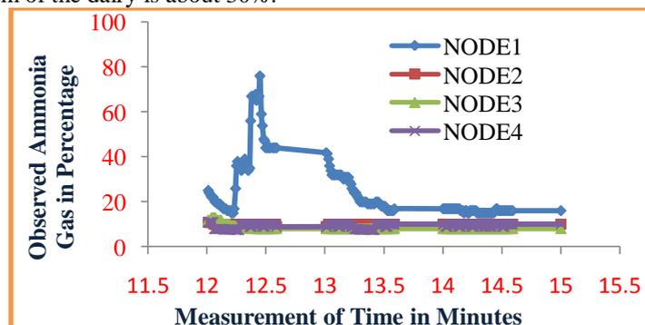
Figure 17 The Graph of Ammonia Gas (NH<sub>3</sub>) values Measured at Refrigerator Section against time in minutes
