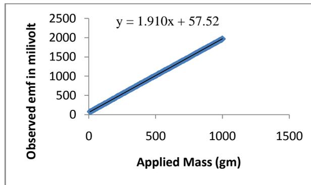
Figure. 8 Graph of observed emf  $V_L$  (mV) against applied mass (gm).
