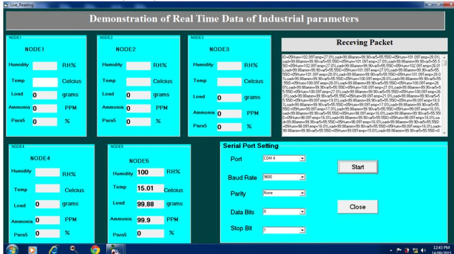
Figure.5 Snapshot of VB Based GUI for Live Monitoring
