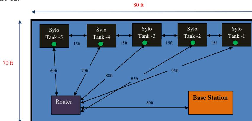
Figure.11 Schematic representation of WSN established at chilling and processing plant of the dairy
