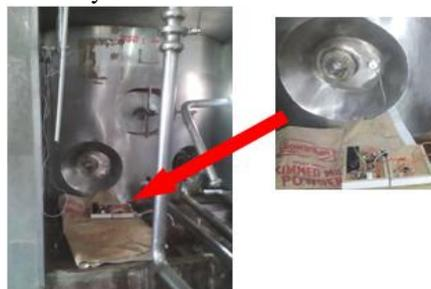
Figure 10 Wireless Sensor Node placed at Tank-5 for measurement of temperature
