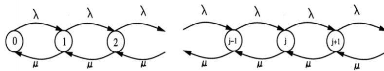
Figure II.2: state transition diagram for an M/M/1 queue model. Adopted from [2]
