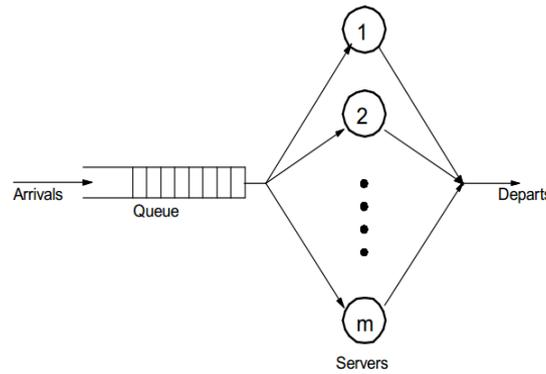
Figure III.1.  $M/M/m$  queuing system with equal service rate. Adopted from [3]
