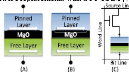
Fig. 2. Illustration of an MTJ and STT-RAM cell.
