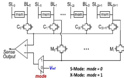
Fig. 3. Reconfigurable extreme mode (X-mode) memory circuit.
