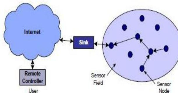
Figure 1. Sensor Network Architecture
