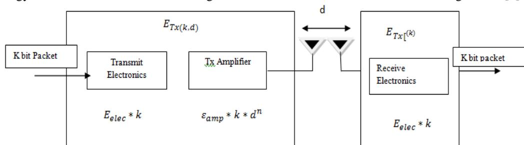
Fig: 1 Radio Energy Dissipation Model
