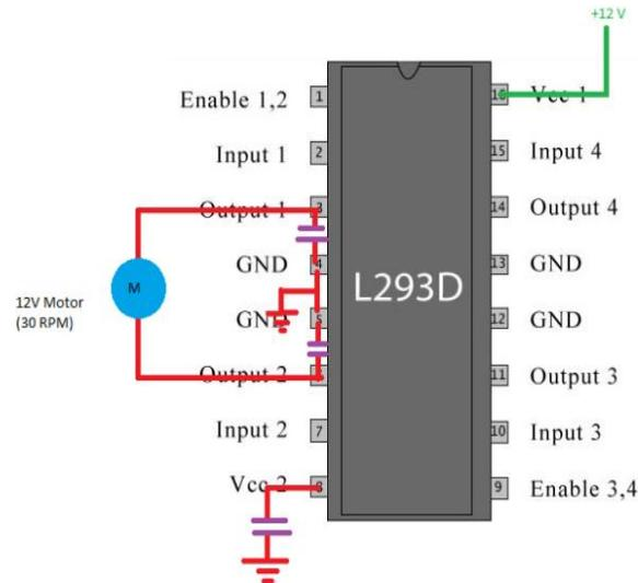
Fig. 3 Driver circuit
