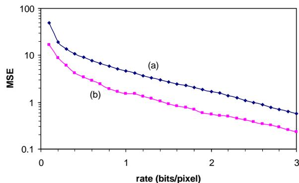
Figure 0-1: Rate Distortion Performance on Transposed Version of coastal\_b7 Test Image Using (a) Integer ACO scheme, Fixed-Rate Compression (with UseFill=1),  $S=16$ , and (b) Float DWT, Full-Frame ( $S=16384$ ) Compression
