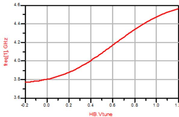
Fig. 8 Simulation result for output frequency versus tuning voltage.
