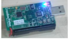
Fig-8: Telosb mote installed with BlinkToRadio application
