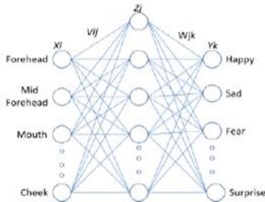
Fig 5: Design of feed-forward back propagation neural network
