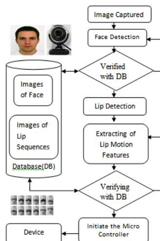
Figure 1: Implementation Block Diagram
