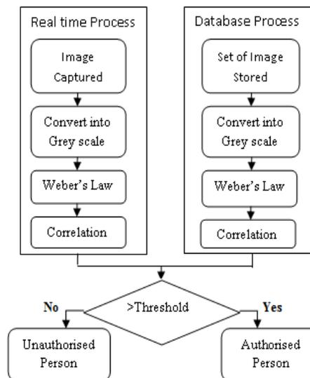
Figure 2: Flow of Face Recognition Technique
