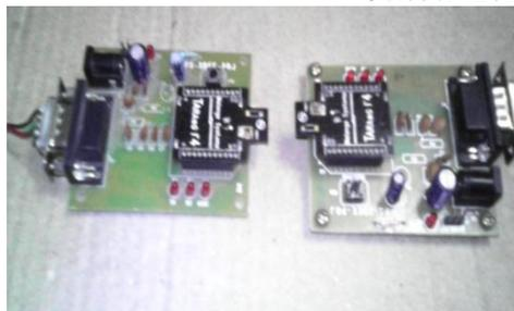
Figure 7: Zigbee Module
