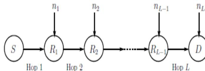
Fig. 2. System model for a multihop wireless link, where SN  $S$  sends message to DN  $D$  via  $(L - 1)$  intermediate RNs.
