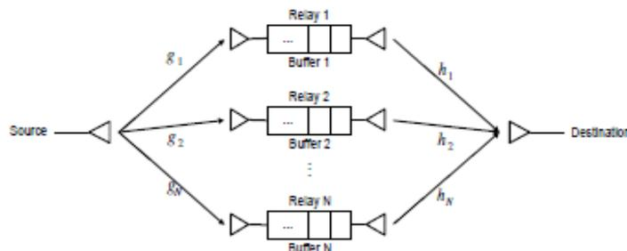
Fig. 4. Relay network with one source, one destination, and N relays where each relay is equipped with a buffer.
