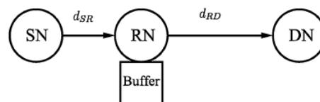
Fig. 5. System model for a buffer-aided three-node network, where SN sends messages to DN via RN.
