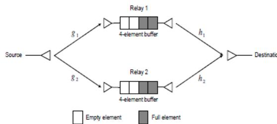
Fig. 3. Relay network with one source, one destination, and two relays where each relay is equipped with a four-element buffer.
