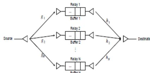
Fig. 9. Relay network with one source, one destination, and N relays where each relay is equipped with a buffer.
