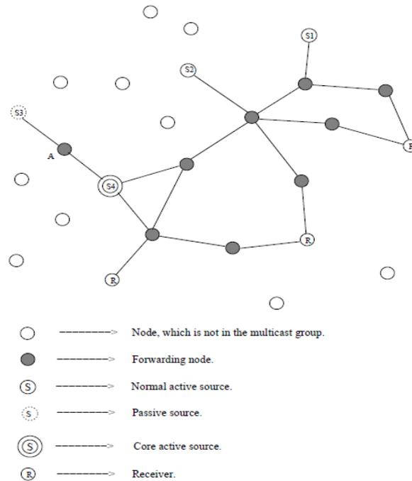
Fig 2 Mesh Topology in DCMP
