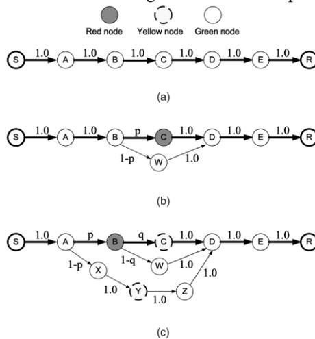
Fig. 1. Use of Bypass to Reduce Congestion
