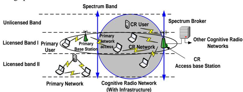
Figure5. Infrastructure-based CR network architecture
