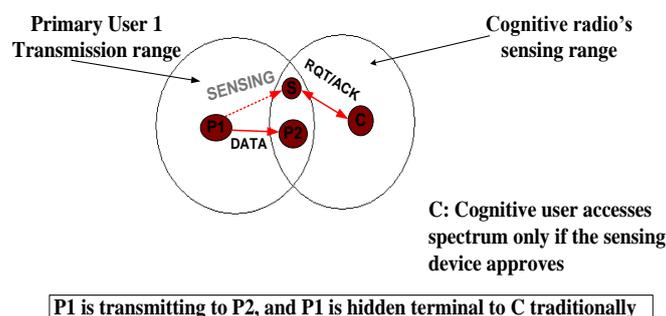
Figure9. Solution of Hidden Terminal Problem by Proposed Sensing Devices
