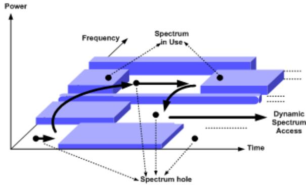
Figure2. Spectrum hole concept
