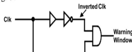
Fig. 5 Circuit for generating warning window from clock signal
