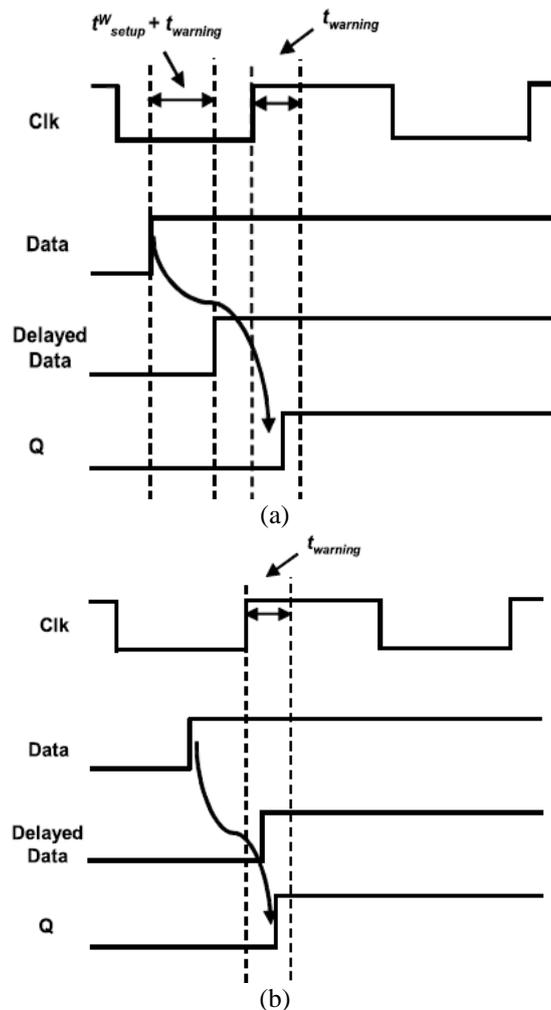
Fig. 1. Proposed warning detection using the delayed data showing the warning window after rising edge of the clock. (a) Early data arrival. (b) Late data arrival.
