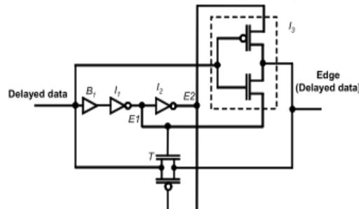
Fig. 4 Pass-transistor-based edge detector.
