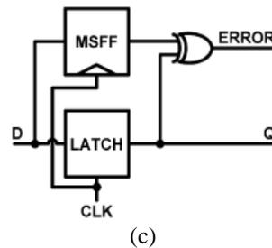
Fig. 3 Error-detection sequential circuits: (a) Razor flip-flop (RFF), (b) transition detector with time borrowing (TDTB), and (c) double sampling with time borrowing (DSTB). CLK is duty-cycle controlled to satisfy min-delay requirements.
