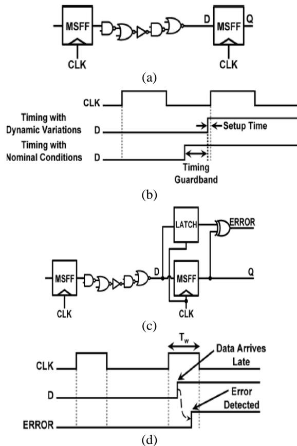
Fig. 2 (a) Conventional path design with (b) conceptual timing diagrams for worst-case dynamic variations and nominal conditions. (c) Resilient path design [5]–[9] with (d) conceptual timing diagram for late arriving input data.
