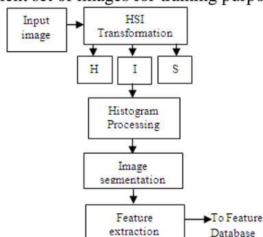
Fig 2: Block diagram of Image analyzer
