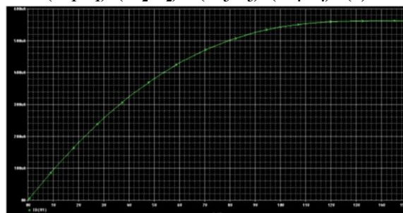
Figure 4. Output curve of a cascode current mirror
