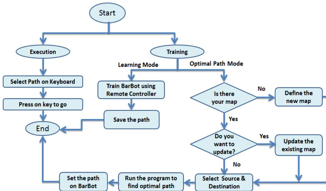
Figure 2. The operational procedure of BarBot.
