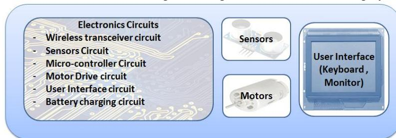
Figure 1. The different parts of BarBot.
