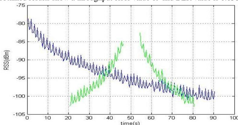
Figure 3: Signal Strength for WiMAX and WiFi Network
