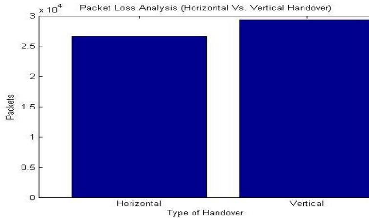
Figure 14: Packet Loss Analysis (Horizontal Handover Vs. Vertical Handover)
