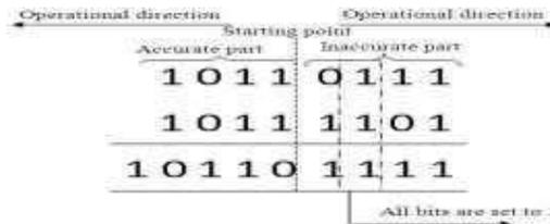
Fig. 1: Arithmetic procedure for 8 bit error tolerant adder
